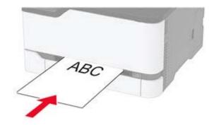
• Load letterhead with the printable side facedown and the top edge entering the printer last for two-sided printing.
